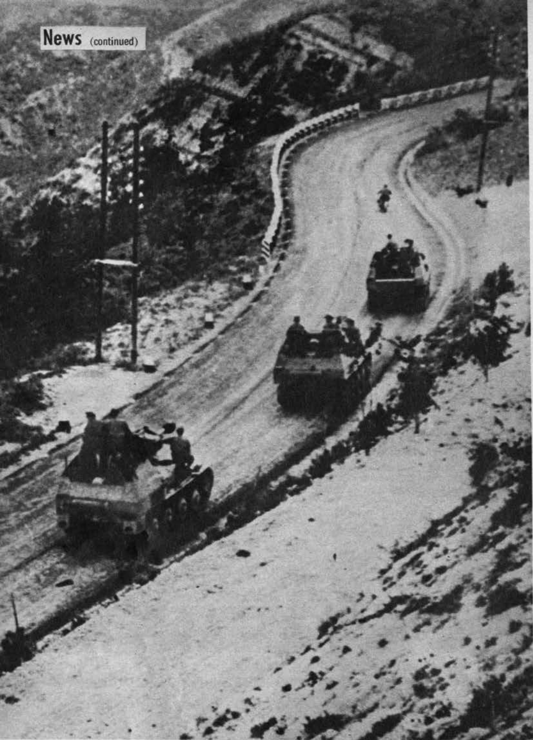
Nazi SP 75-mm. guns on the PzKw 38 chassis cross the Brenner Pass. This aerial view shows boxlike, open-topped crew compartment with sloping sides cut down at the back.
